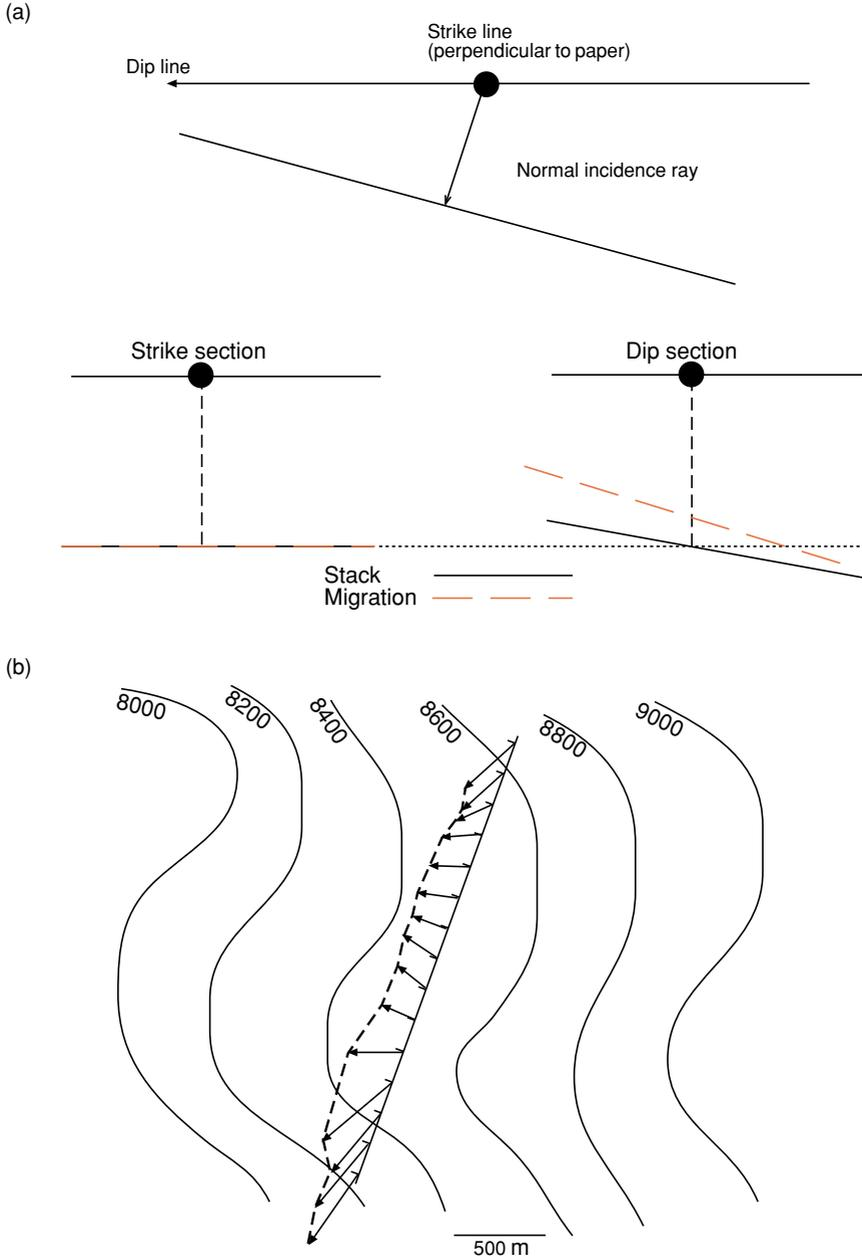
**Fig. 1.3** (a) For a 2.5-D structure, dip and strike lines do not tie after migration; (b) map view of reflection points for a 2-D line (contours are depth in feet (ft)).
